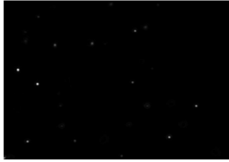
Fig. 2 Example of an optimal image to allow accurate particle centering by NTA
